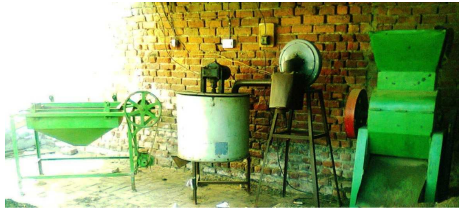
Figure 1: Mechanical Dryer for Bioslurry
